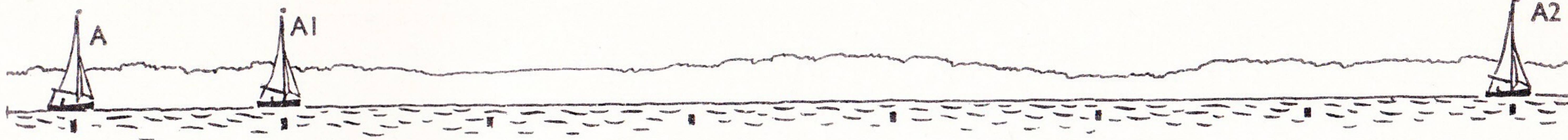
Fig. 39 With the current. A boat moving at 4 knots with a 3-knot current will make 7 knots (A to A2)
