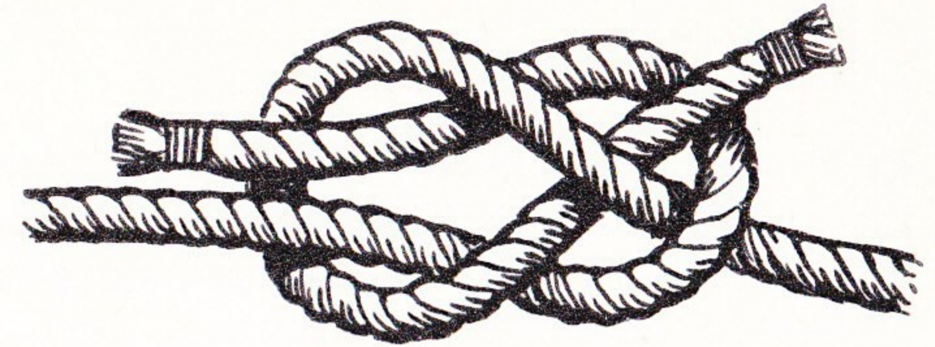
Fig. 53 Sheet Bend. For tying two ropes of the same size together or attaching a rope to a loop.
