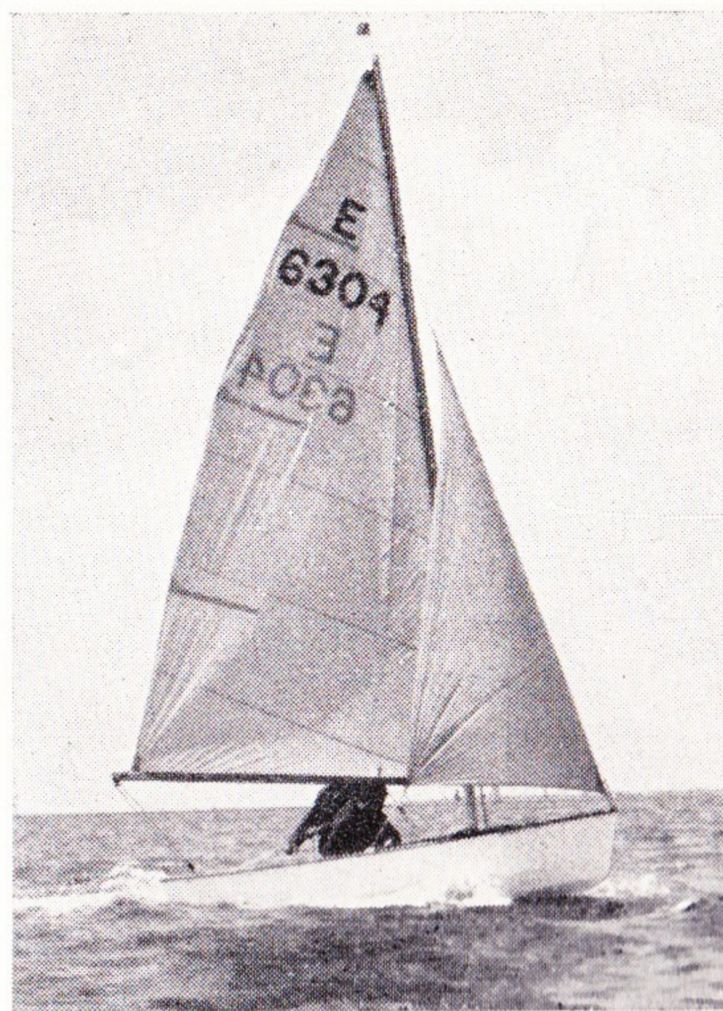
Fig. 11. National Enterprise showing chines at the bow
